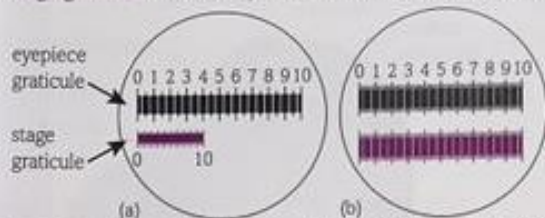
Figure 1 Eyepiece graticule and stage graticule at (a) \times 40 magnification, and (b) \times 100 magnification.
